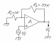
(5pts) a) Determine the 3dB frequency,  $f_{3dB}$ , for the non-inverting amplifier.
